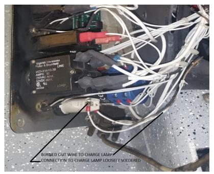
Fire damage. Note the burned-out wire running to the charge lamp, and the missing screw to the charge lamp replaced with a loose solder blob on the wire.
